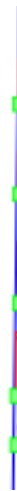
FIG. 2 – A simple column model. The red rectangles are bounding boxes for connected components, the green dots are the reference points used for each bounding box, and the blue line is a robust linear fit to the reference points.
